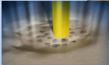
The fact that the TFN's are placed into the scour hole below the surrounding seabed level and the sediment is trapped within the tyres means that the problem of 'Secondary Scour' and the scour protection moving away from the turbine pile is eliminated.
