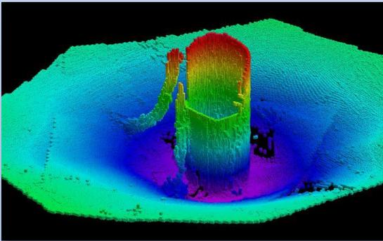
These holes around the turbines create a number of problems for the operation of the windfarm as there is a longer exposed length of the turbine piles and less penetration depth into the seabed.
